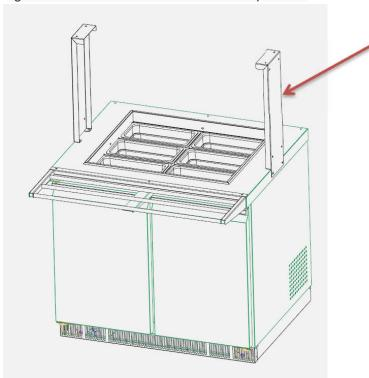
3. Place the upper bracket on the left and right brackets and align the mounting holes for the upper bracket and the left and right brackets
