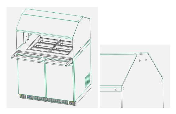
7. Use the L shape connector to connect the top cover and side panels, totally 4 corners as showed in below image, use screws and nuts to fix them in place.
