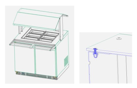
6. Install the side panels to the mounting holes of the left and right brackets. Align the Sneeze Guard and tighten the screws.
