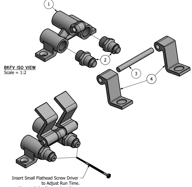
to Adjust Run Time. Turn Left for Shorter Run Time. Turn Right for Longer Run Time.
